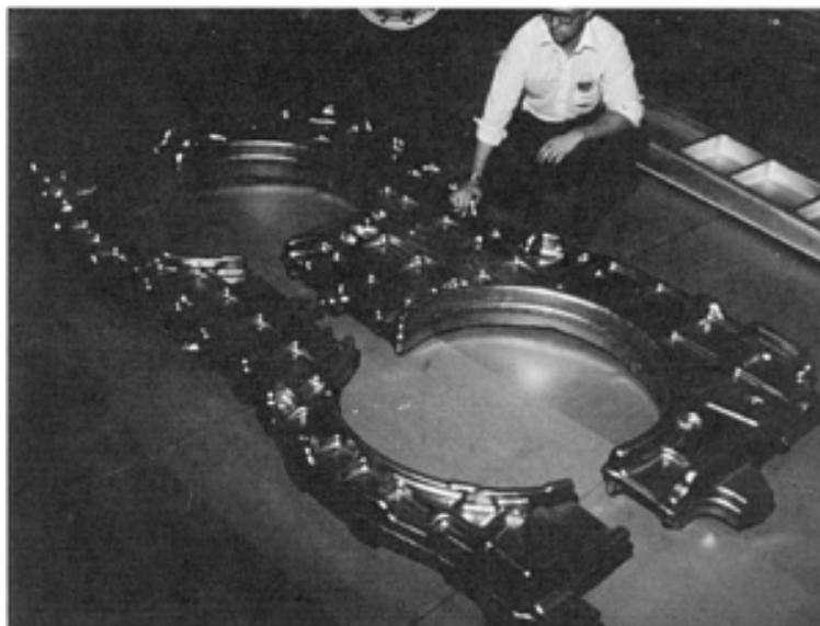
Fig. 12 Alloy Ti-6Al-4V forgings for upper and lower bulkheads used on the F-15 that were produced on a 450 MN (50,000 tonf) hydraulic press using conventional forging methods.
