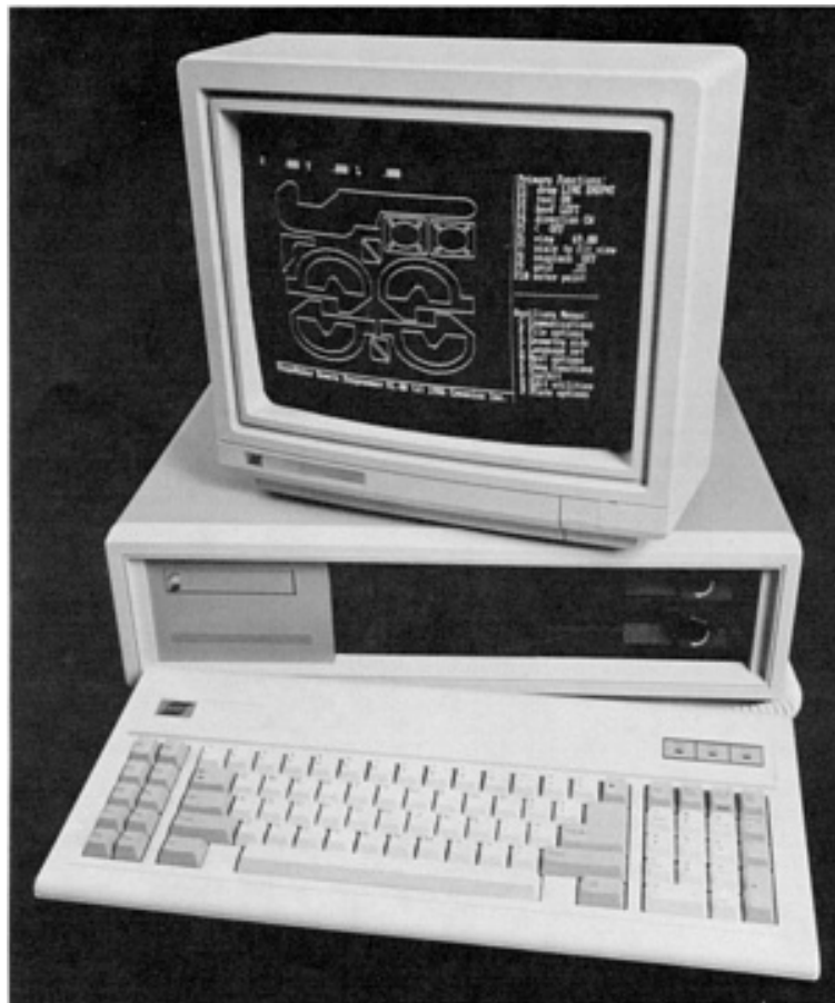
Fig. 8 Parts programming system for nesting of shapes. Layouts of part patterns can be performed on-screen using such a system, resulting in optimum material use. Courtesy of ESAB North America, Inc.
