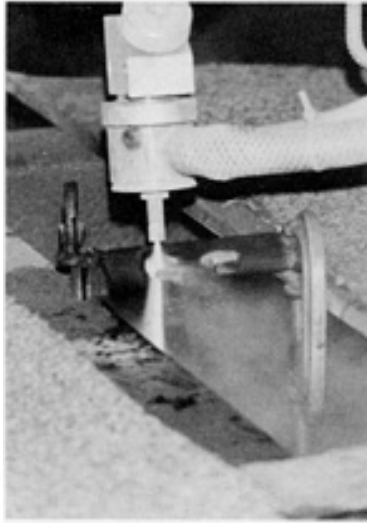
Fig. 6 Stationary waterjet nozzle cutting through a movable workpiece (René 100 alloy gating contacts). Courtesy of Department of Industrial and Manufacturing Engineering, University of Rhode Island.
