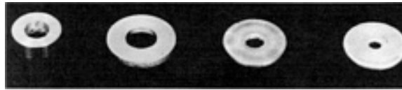
Fig. 14 Variation in shape of ring test specimens deformed the same amount under different frictional conditions. Left to right: undeformed specimen; deformed 50%, low friction; deformed 50%, medium friction; deformed 50%, high friction.
