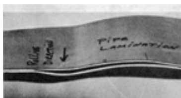
Fig. 29 Laminations in rolled steel sheet resulting from insufficient cropping of the pipe from the top of a
