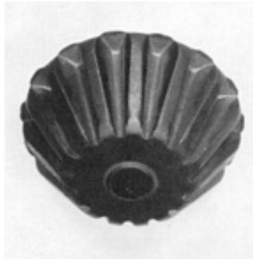
Fig. 44 Warm precision forging of a 1.25% C UHC steel billet into a bevel gear. Forging temperature was 650 °C (1200 °F).
