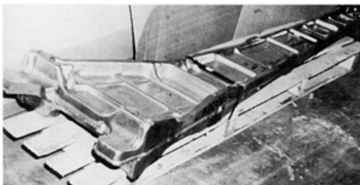
Fig. 6 Titanium alloy wing spar forged in a closed-die using \alpha - \beta and \beta forging techniques. The part is 2.8 m (110 in.) long and weighs 262 kg (578 lb).
