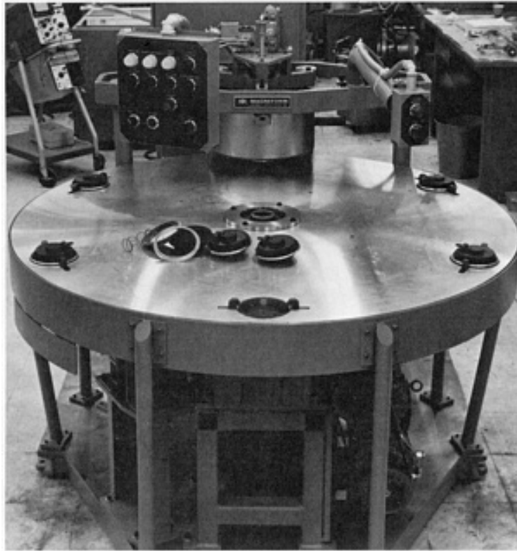
Fig. 5 Semiautomatic EMF system for assembly of automotive cruise control power units.
