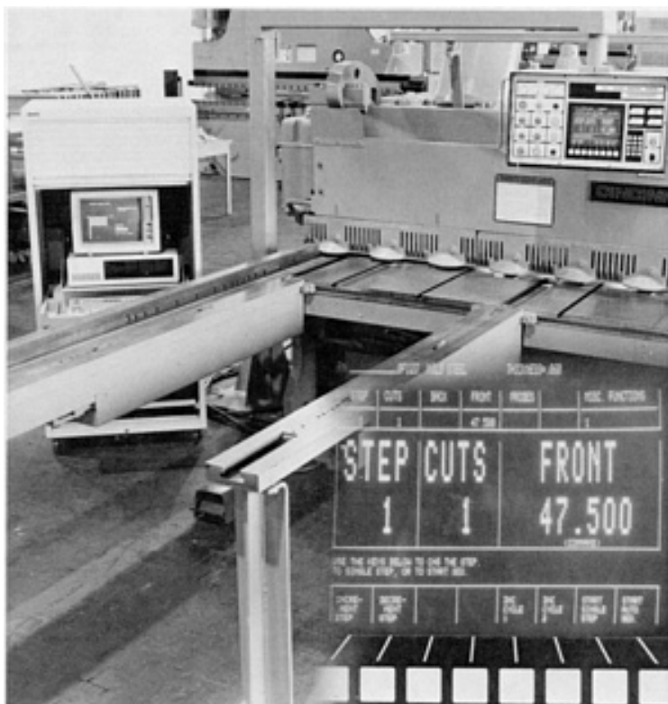
Fig. 4 Microprocessor-controlled shearing machine, with inset (lower right) showing LED display. Courtesy of Cincinnati Inc.
