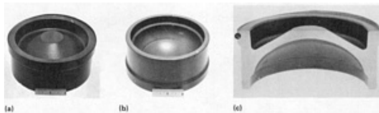
Fig. 45 Aft closure, for a guided missile, that was superplastically formed at 815 °C (1500 °F) from a 1.6% C UHC steel. The processing procedure consisted of warm pressing (800 °C, or 1470 °F) liquid-atomized powders into a billet and forging the resulting billet into plate. The plate was then superplastically formed to the final shape (a and b). (c) Cross section of the part
