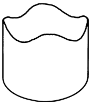
Fig. 3 Drawn cup with ears in the directions of high r value.
