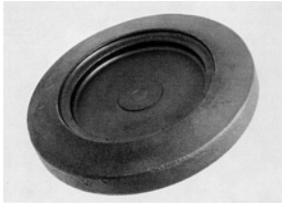
Fig. 1(b) Differential bevel gear weighing 3.5 kg (7.8 lb) that was hot forged from 16CD4 (similar to 4130) bar material on a 24 MN (2700 tonf) horizontal forging machine. Courtesy of National Machinery Company.
