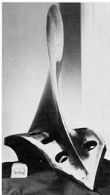
Fig. 2 Forged and machined alloy 718 marine propeller blade. Courtesy of Ladish Company
