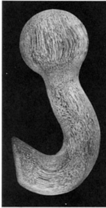
Fig. 7 4140 steel forged hook showing fibrous structure (flow lines) resulting from hot forging. Etched using 50% hot aqueous HCl. 0.5×
