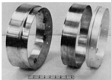
Fig. 20 Aluminum alloy engine inlet mounting assembly for an aircraft before (right) and after (left) assembly by electromagnetic forming. Courtesy of Grumman Aircraft Systems
