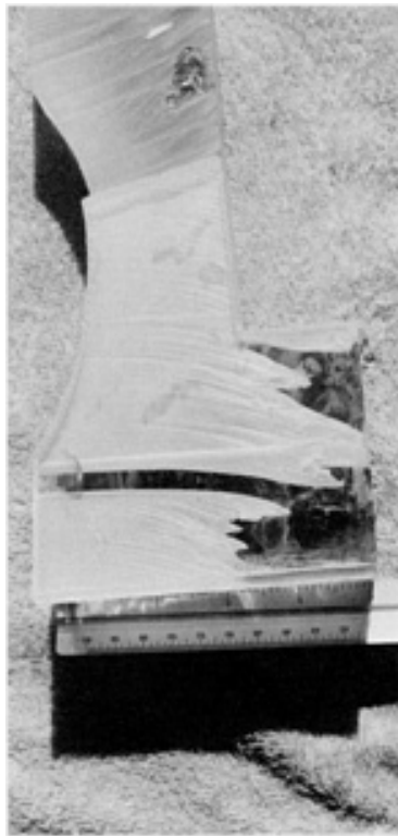
Fig. 14 Bending of kerf in a Plexiglass workpiece subjected to excessively high traverse cutting speeds. The portion at the bottom was pierced before cutting, and this caused a section of the hole to be eroded away as it was subsequently cut by abrasive waterjet nozzle. Courtesy of Department of Industrial and Manufacturing Engineering, University of Rhode Island.
